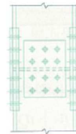
Bolt Connection (on-site)
